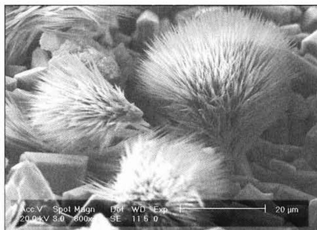
Figure 4. Acicular sprays of connellite on atacamite. Magnification,x800. Field of view = 0.08mm.
